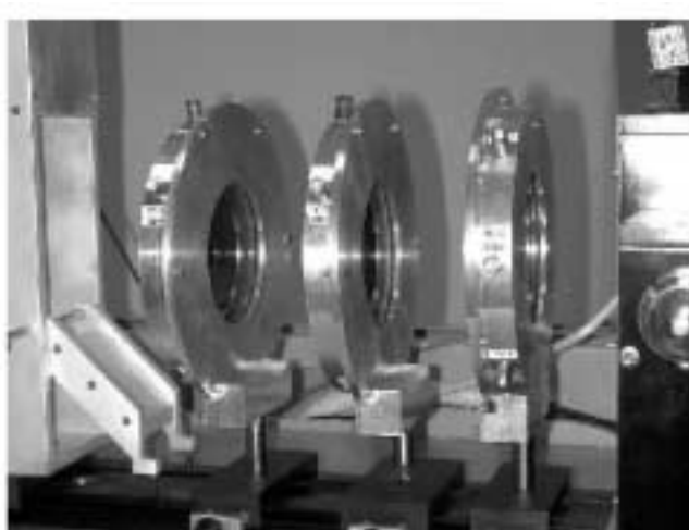
Figure 3: A view of the two monitor chambers and four sectors chamber on the CATANA line.
