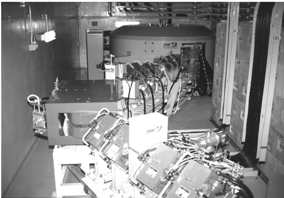
Fig. 1 cyclotron and part of beam transport line
